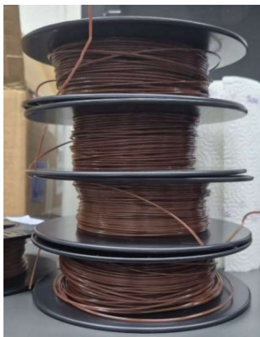
Figure 1. Filaments of COC/Cu composites.
