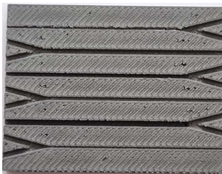
Figure 1. Microreactors 3D printed of 17-4 PH composite material
